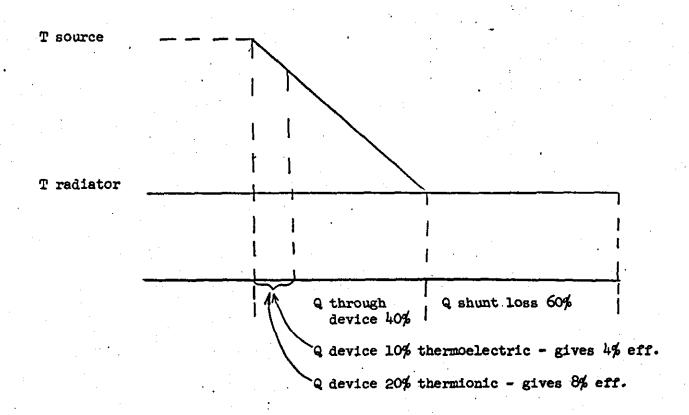
Figure I is a plot of the thermal efficiency of a system. On the left we plot the temperature of the source and the temperature of the radiator. The distances along the bottom are the Q representing the heat dissipation through the device and the Q for the shunt loss or the loss of heat by-passing the device.
