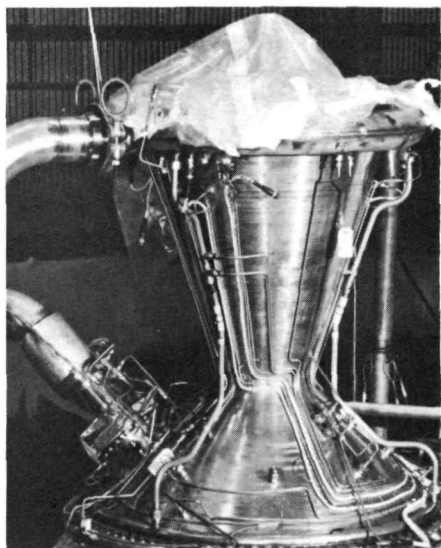
A nuclear rocket nozzle under construction, showing coolant tubes welded to the basic bell-shaped structure.
