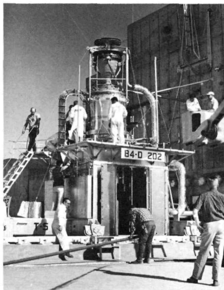
Moving a Kiwi reactor from its assembly bay to a test cell. This "Jackass & Western RR" locomotive can be remotely controlled.
