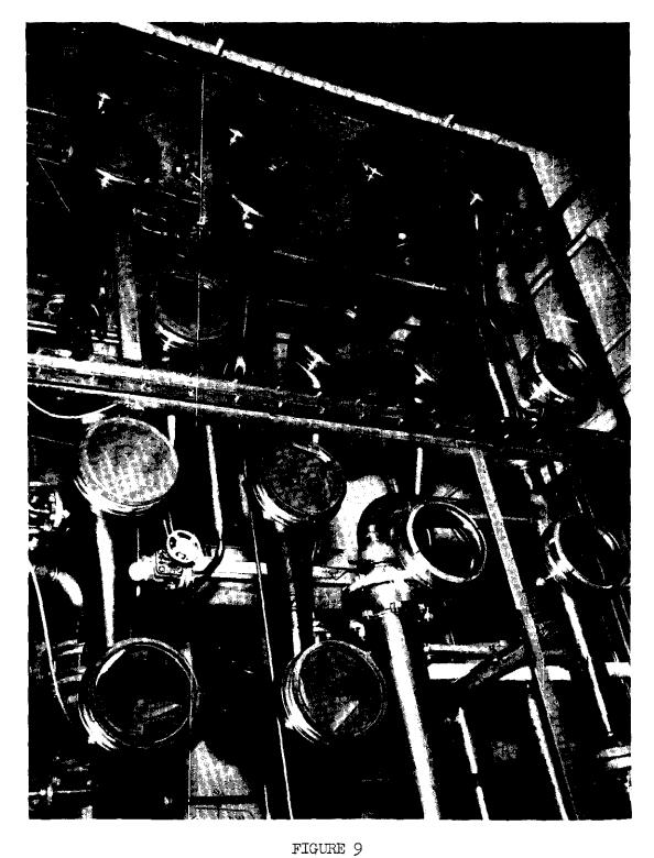
Anion Exchange Hood Showing Concentrator and Condenser
