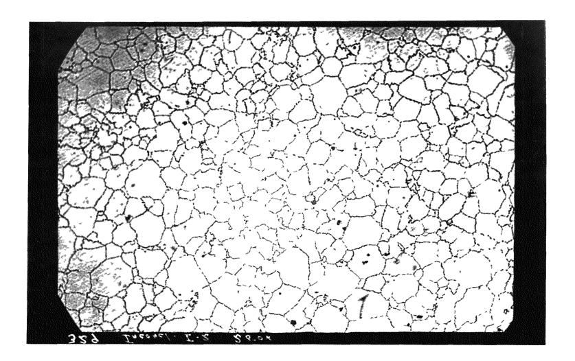
Figure 2. Photomicrograph of stock Inconel window surface. Magnification 250.
