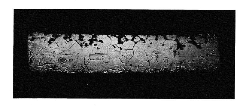
Figure 4. Photomicrograph of Inconel window cross section. Run No. 1: irradiated and heated. Deuterons impinged on lower surface. Fused fluoride was in contact with upper surface. Magnification 250.
