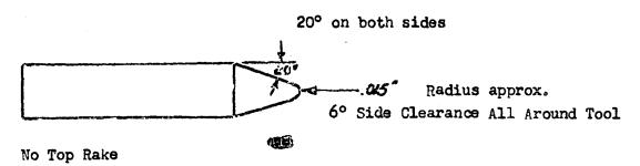
This enables tool to cut in both directions.
