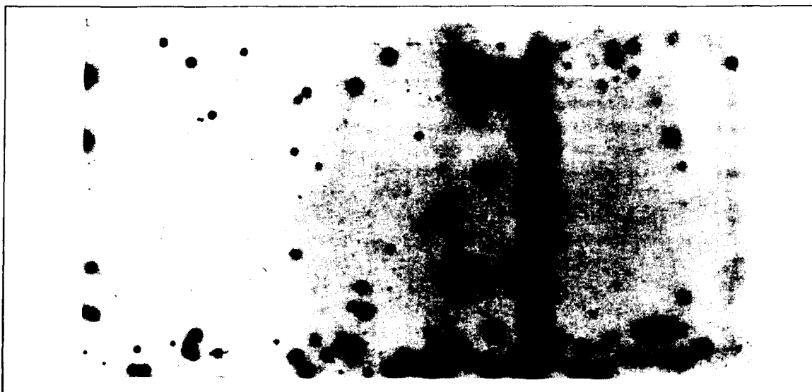
Fig. 26 Autoradiograph of fallout plate 300 meters downwind.
