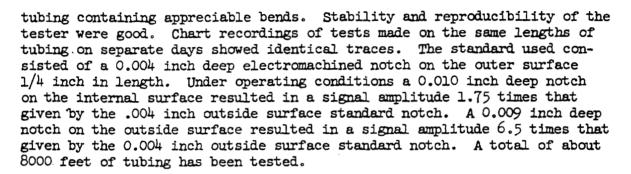
Based upon observations of the eddy current test signal indications, estimates were made as to nature of the tubing irregularities. The tubing specimens were then destructively examined by Physical Testing. Estimates and corresponding destructive examination results are as follows:
