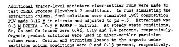
Engineering Studies - The first pilot plant tests of the CSREX process was made during the month with favorable results. This process employs a mixture of 0.5 M BAMBP and 0.3 M DZEHPA in Soltrol-170 to co-extract cesium, strontium and rare earths. The cesium and strontium are stripped from the solvent with dilute nitric acid (0.05 M) followed by rare earth stripping with 0.5 - 2 M nitric acid. The process is quite similar to the DZEHPA process and would use the same equipment.
