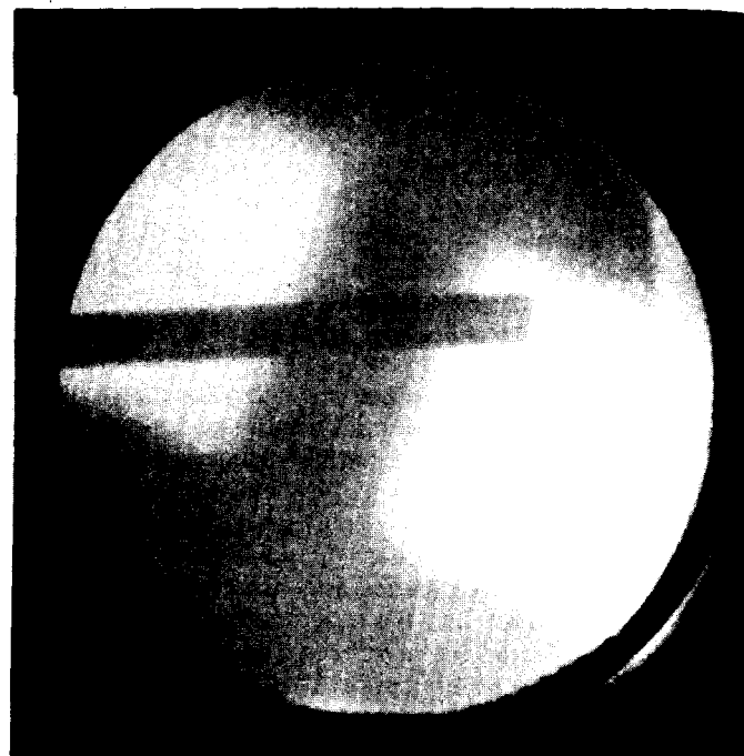
Fig 2 Soft x-ray micrograph taken at beamline 3-4. Sample is 2000 line/inch nickel mesh suspended inside emitter. Two of the roughly 8 micron openings are visible. Tip radius is approximately 15 microns. Voltage on emitter is 18 KV. The horizontal bar is the x-ray beamstop held in front of the detector. The resolution of this image is estimated to be 3000-4000 \text{\AA} .
