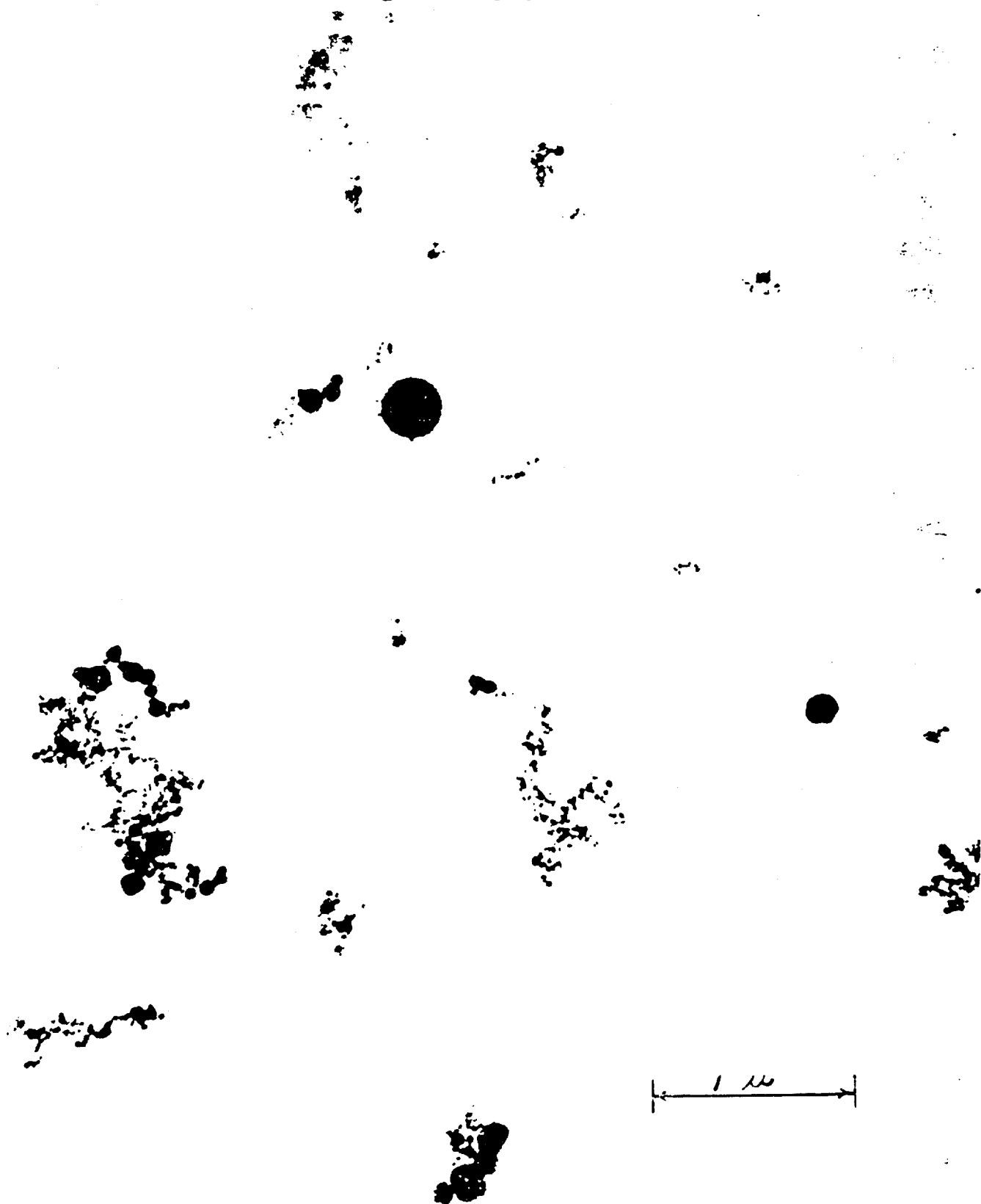
Figure 5. Electron micrograph of a uranium dioxide fume produced at a concentration level of 80.7 \text{ mg/m}^3
