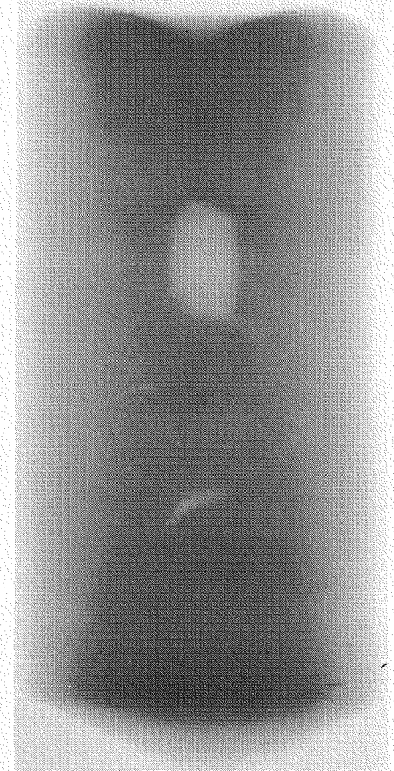
Yttrium ingot vacuum melted in molybdenum crucible and cast into cooled copper mold
